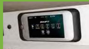
Integrated DAB and FM radio tuning and sound setting control (part of Swift control system)
